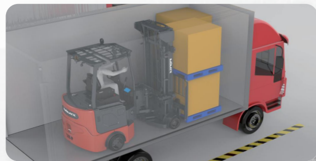
Low mast design enables handling inside containers
