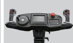
The OPS pedal and left and right side armrests have an in-place sensing function. Armrests and pedals can both guard the operators' safty that the truck can only be operated when a person is in position.
